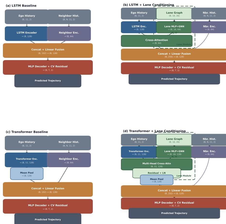
Figure 2. Architecture overview of the four model variants. Left column: baselines without lane information. Right column: lane-conditioned variants with the lane conditioning module (green dashed box) added as a modular plug-in. The LSTM variants (top row) use single-vector cross-attention pooling, while the Transformer variants (bottom row) use multi-head cross-attention over the full ego sequence to capture timestep-level lane–trajectory interactions. Arrows indicate the direction of data flow between modules.
